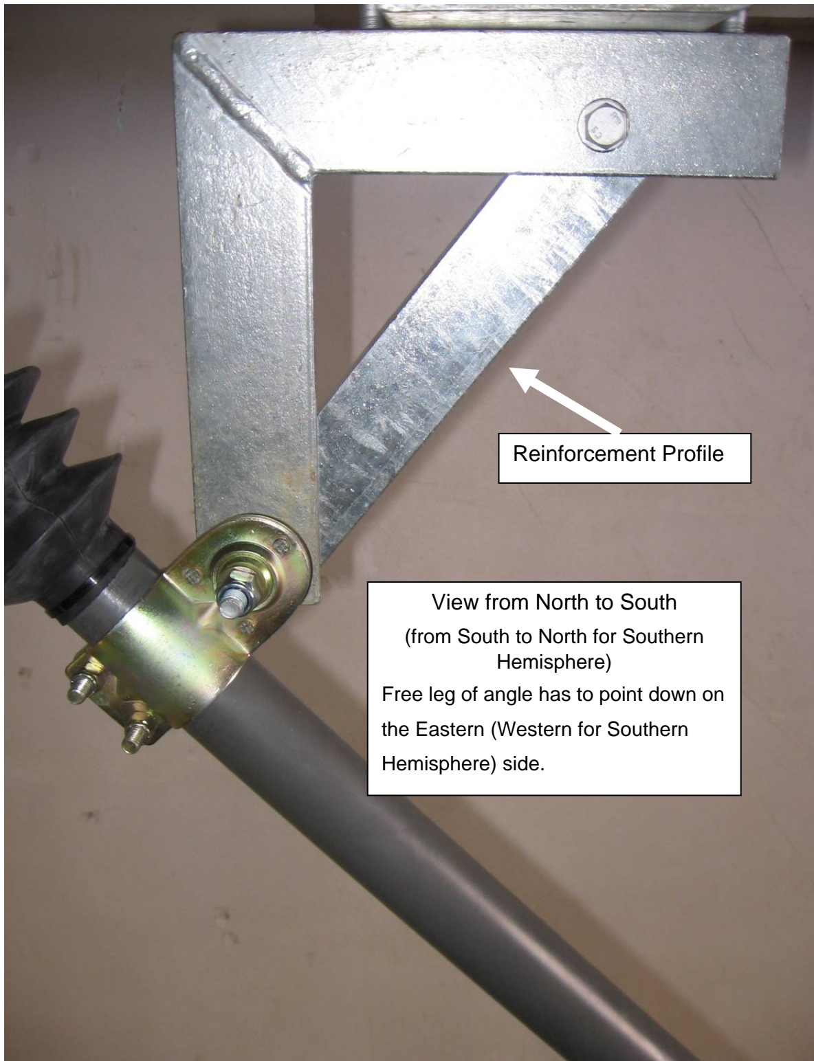
Fig. 5.4 Arrangement of lower motor fixation
