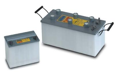
FIAMM's **PMF** battery range can be used in standby mode for long discharge rates or for cycling applications. Its tubular positive plates with low antimony together with lead-calcium negative plates guarantee an unsurpassed cycle life and a long life even in the worst operating conditions.
