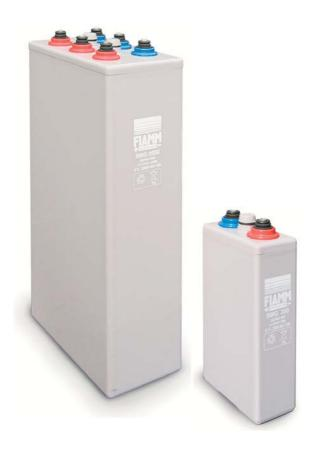
The FIAMM **SMG** range of valve regulated lead acid stationary batteries combine the benefits of recombination technology (i.e. virtually no maintenance due to very low gas emissions) plus the advantages of conventional vented batteries with positive tubular plates (i.e. long life and excellent cycling capability).
